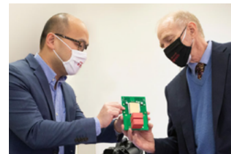
Professor Fang Luo, PhD, and Spellman C.E.O. Loren Skeist, MD, inspect a 3D integrated high-voltage GaN power module that Luo fabri- cated for electric vehicles.
