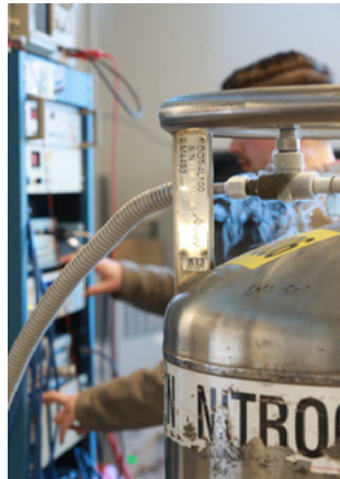
Cryogenic testing of GaN modules
