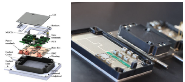
Packaging of wide-band semiconductor inverters developed at Spellman High Voltage Power Electronics Laboratory
