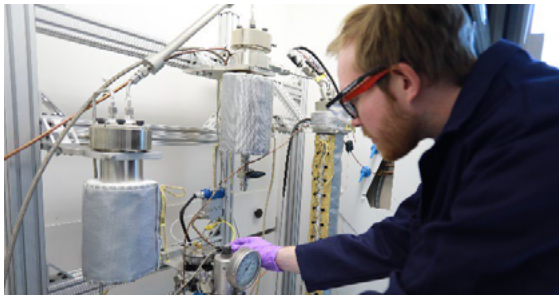
Development of prototype gas negation unit at IGIT facility
