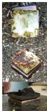
Figure 1 Top: fresh gel Middle: charring while burning Bottom: char after 3 min of burning
