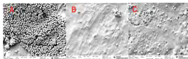
Figure 3. Biomineralization Image captured by Scanning Electron Microscopy on Day 28 of DPSCs from A)NT Thin Films B)NT Thick Films C)T Thin-Thick Films
