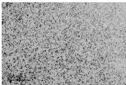
Fig. 2: Top-view TEM micrograph of assembled AuRu NPs at surface pressure of 2 mN/m.
