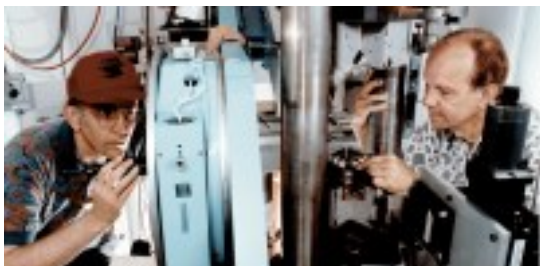
Don Weidner and Mike Vaughan working to install SAM-85 on the superconducting wiggler beamline [X17B2] at NSLS.
