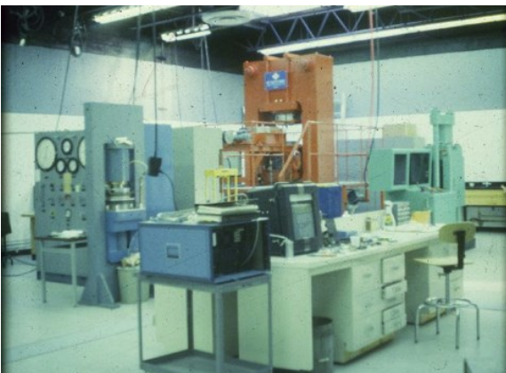
The High Pressure Laboratory in 1986 with the USSA-2000, the 500-ton Harwood press with girdle-anvil and the 1000-ton Kennedy-Getting press installed and operational.
