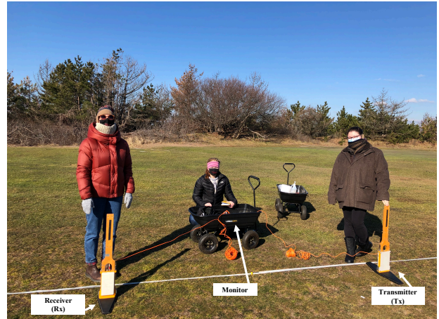
Figure 4. Data acquisition at X=23 grid line at the RMSP golf course. CMP setup using 400 MHz bistatic unshielded antennas.
