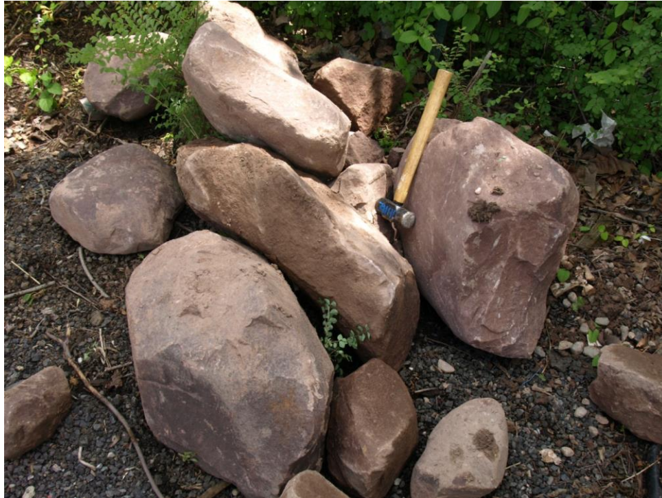
Figure 3 – View of subangular boulders and cobbles of Passaic Formation siltstone and sandstone mucked from base of Shaft #23. Note the tabular aspect of the boulders, a relic of original bedding, and the incipient polishing by mechanical means. Hammer is 38 cm (15”) in length. (Dukelabs digital image taken 14 June 2013.)
