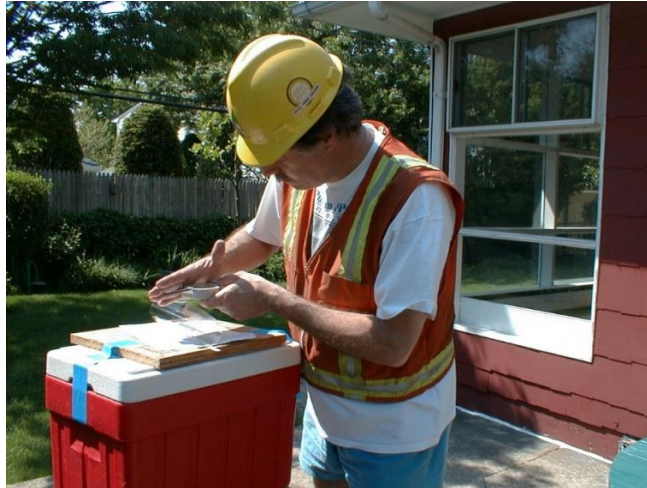
Figure 20 – Strike and dip of planar features were remeasured by sighting and compared to tunnel measurements from rolled map mylars aligned with respect to true north using a Brunton compass outdoors. Liquid refreshments stored in the cooler were enjoyed after the measurements were made, compared to map data and recorded.
