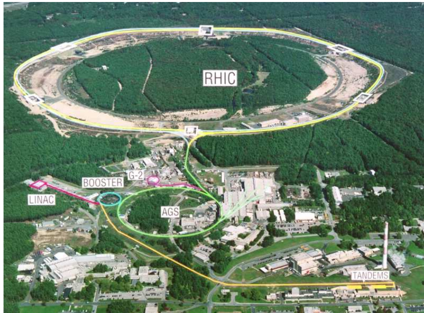
Figure 2.1: An aerial photograph of the RHIC facility. The various colors show different facilities that produce the ion beams and bring them up to full energy. The main RHIC rings are the yellow and blue lines as shown.
